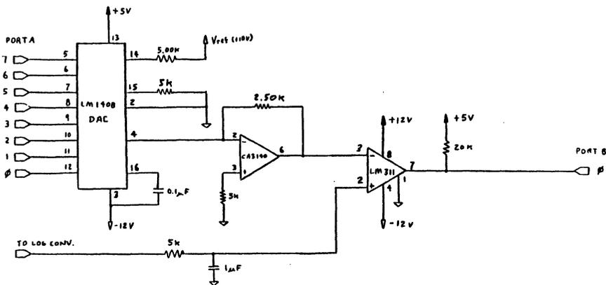
Figure 6. ANALOG TO DIGITAL CONVERTER
