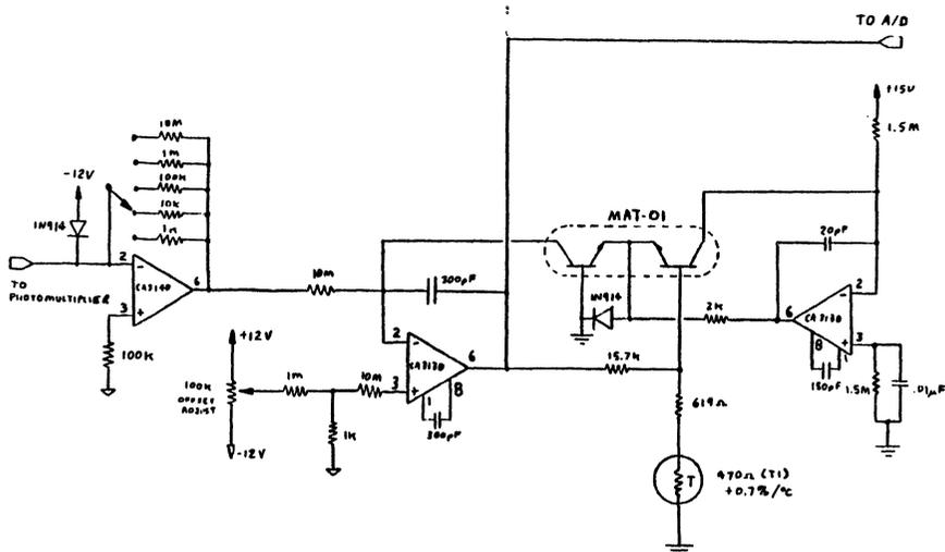
Figure 5. AMPLIFIER AND LOG CONVERTER
